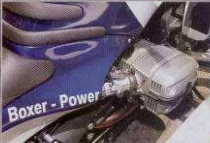
BMW's liquid-cooled, fuel-injected 1150cc boxer twin propels the GG with impressive force and refinement.
