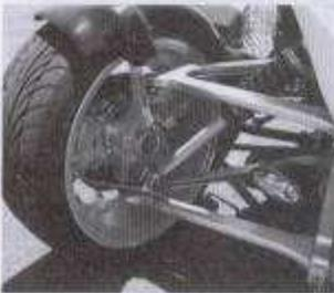
The hubs and steering arms at each corner are billet aluminum works of art, attached to equally gorgeous milled alloy carriers.
