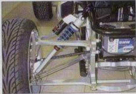
To affix dual A-arms to the front of the BMW motorcycle, an aluminum bulkhead bolts to the frame in place of forks. From there, the inlet arms connect to a billet spindle upright. Steel tie-rods turn the wide, low-profile tires.
