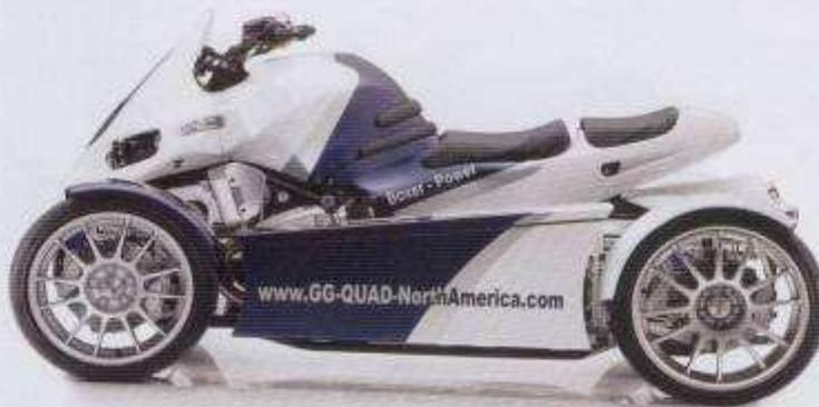
Sitting on the GG Quad, one immediately feels at home as a motorcyclist; the controls and ergonomics are straight from a two-wheeled machine. At the same time, the four-wheel-derived stability at a standstill is noted, freeing the rider from satisfying the requirements of balance. The start button fires the fuel-injected 1130cc boxer motor instantly, and the BMW motor's reassuring vibration informs the rider that it is time to engage the six-speed manual transmission.
