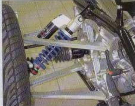
An aluminum differential housing rests where a floating swingarm should. Standard CV-joints transfer power to the outer corners. A coil spring shock offers complete adjustment for varied road conditions. Floorboards are provided for the passenger only.
