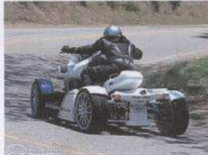
The different dynamics of riding the GG Quad are readily apparent in cornering, with counter-steering and powerslides not an option.
