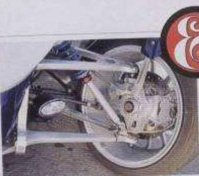
» The GG Quad's billet-machined front suspension shows incredible attention to detail.
