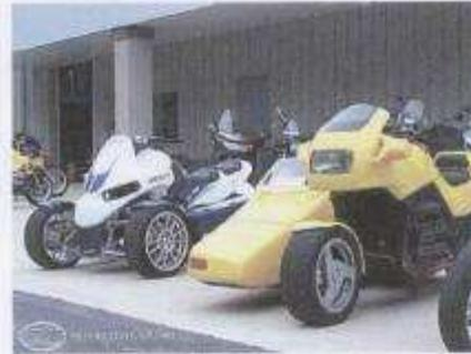
The GG Quad (left) poses next to the yellow GG Duetto sidecar, a former project of G+G's Walter Gruter. It features hub-center steering and a swingarm front end.
